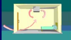
Negative Pressure Room with In-Room HEPA Filtration
